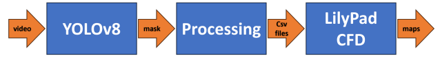
Fig. 1: Proposed pipeline for the automation of the design of our DT in LilyPad.
