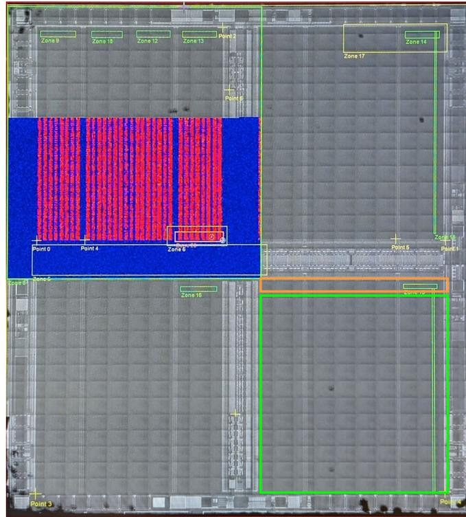
Fig. 7. Laser testing run with chip-enabled test mode of the entire first quadrant, including memory array, supply spines, controlling logic, and periphery interfaces, showing energy and region dependency for SEL occurrence (tested zones highlighted).
