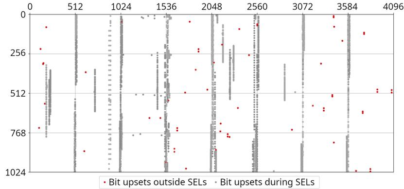
Fig. 5. Logical bitmap of the memory address space with the identified bit upsets during a March C- run with a LET of  $48.5 \text{ MeV cm}^2/\text{mg}$ . The x and y axis represent addresses in an arrangement based on the logical memory organization. For this bitmap, bit upsets during and outside SELs were highlighted in grayscale shades (for distinct events) and red, respectively.
