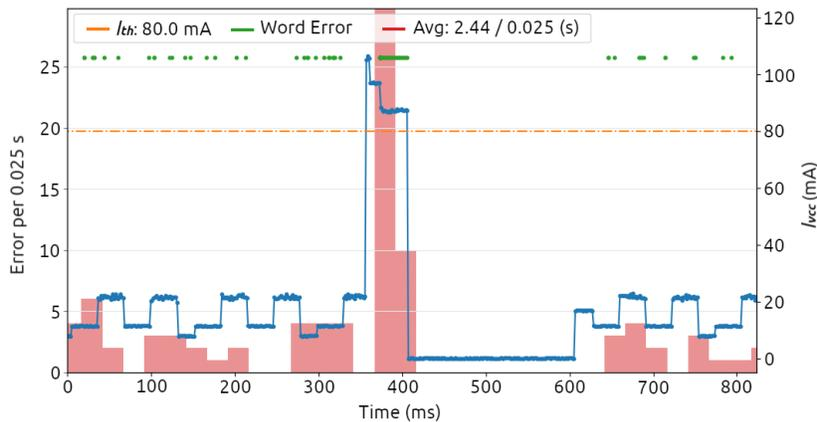
Fig. 4. Example of error rate (bit upsets) variation during SEL events. Test run for a dynamic test (March C-) during heavy-ion irradiation with a  $LET = 14.4 \text{ MeVcm}^2/\text{mg}$ .
