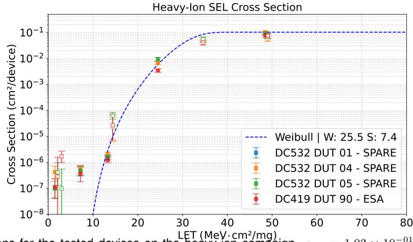
Fig. 3. SEL cross sections for the tested devices on the heavy-ion campaign.  $\sigma_{sat} = 1.03 \times 10^{-01} \text{ cm}^2/\text{device}$  and  $LET_{th} = 7.2 \text{ MeVcm}^2/\text{mg}$ . Test modes included standby, chip-enabled, static, March C-, and Dynamic Stress.
