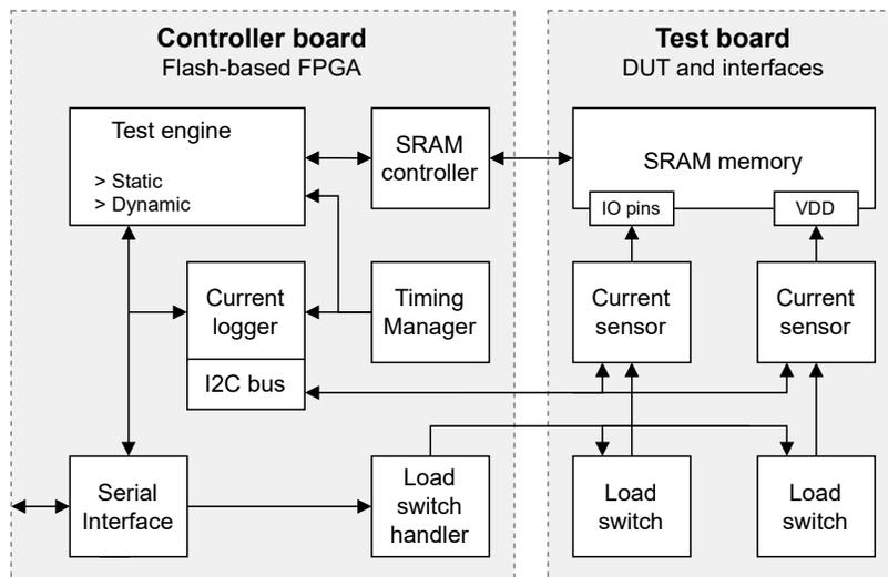
Fig. 2. Simplified diagram of the experimental setup used for the three experiments. The instrument is connected to a host computer through the serial interfaces.
