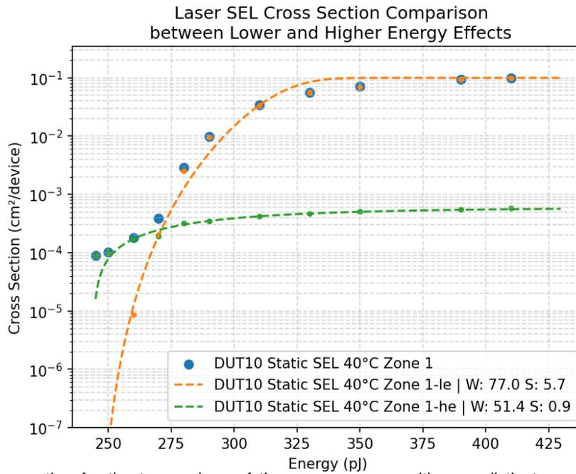
Fig. 8. Static SEL cross section for the two regions of the memory array with very distinct sensitivities. Zone 1-le:  $\sigma_{sat} = 5.88 \times 10^{-4} \text{ cm}^2/\text{device}$  and  $E_{th} = 244 \text{ pJ}$ . Zone 1-he:  $\sigma_{sat} = 9.94 \times 10^{-2} \text{ cm}^2/\text{device}$  and  $E_{th} = 244 \text{ pJ}$ .
