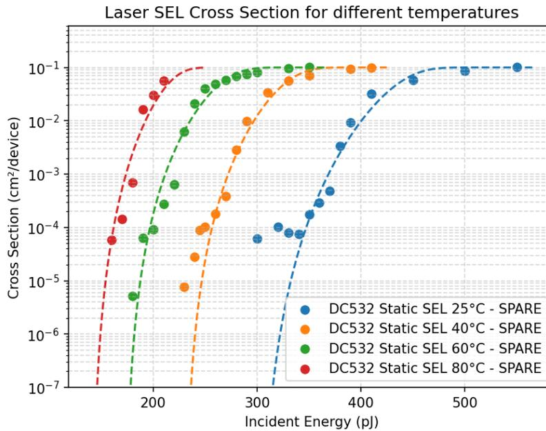
Fig. 9. SEL cross sections for static mode normalized for the entire memory die area using four temperatures: 25°C, 40°C, 60°C, and 80°C.
