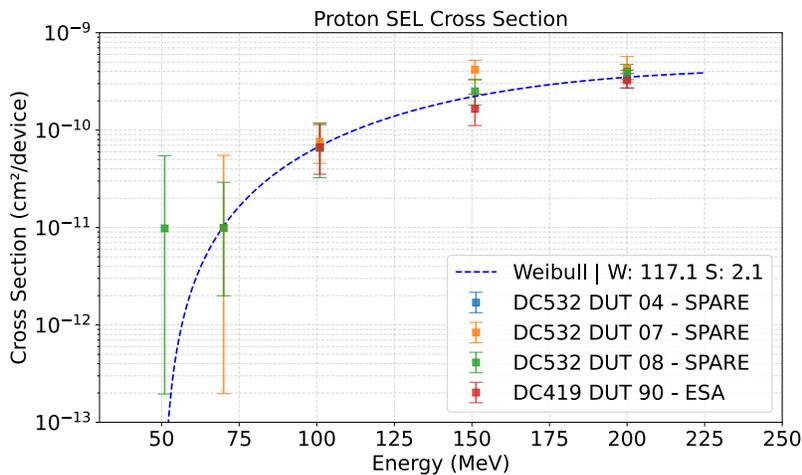
Fig. 6. SEL cross sections for the tested devices on the proton campaign.  $\sigma_{sat} = 4.29 \times 10^{-10} \text{ cm}^2/\text{device}$  and  $E_{th} = 50.9 \text{ MeV}$ . Test modes included static and March C-.
