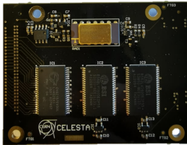
Fig. 1. Radiation monitoring system board of the CELESTA CubeSat [25].
