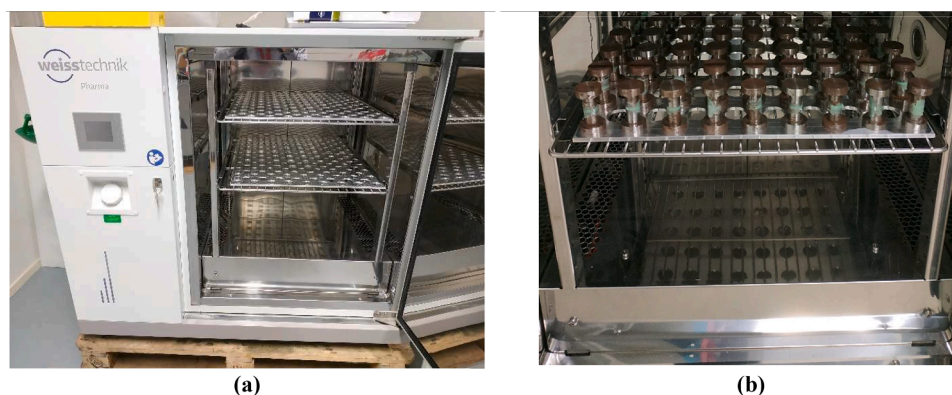
Fig. 5. Climatic oven: a) aluminium plates; b) placement of the adhesive specimens.
