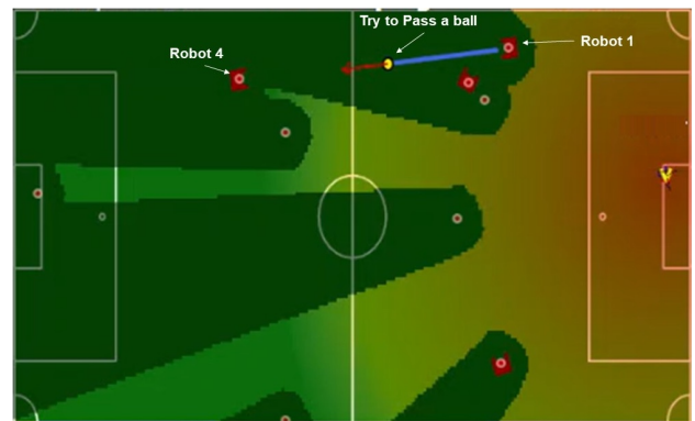
Fig. 4. States of the robots on the field at time k + 1 (Robot 1 has decided to Pass the ball to robot 4)
