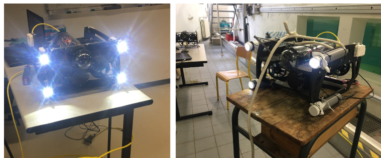
Figure 10. Four LEDs equipped on the follower robot.
