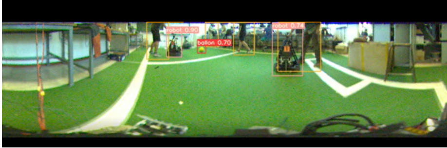
Fig. 1. YOLOv3 for object detection running on a GPU with omnidirectional camera.
