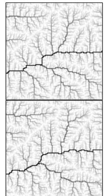
blocks of the lower resolutions (inset, top), with sharp turns. We prevent these artifacts by adding some jittering (inset, bottom) during the upsampling process, where a uniform random offset in  $[-0.25, 0.25]^2$  is added to the locations of the nodes before interpolation.
