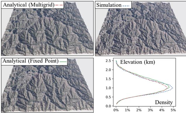
**Figure 5:** We compare our method at steady state (with multigrid, top left) with a simulation [CBC\*16] (top right) and a fixed point algorithm [Ste21] (bottom left). These three methods should produce similar results, which we highlight by comparing their hypsometry (or the density plot of the elevations, bottom right).
