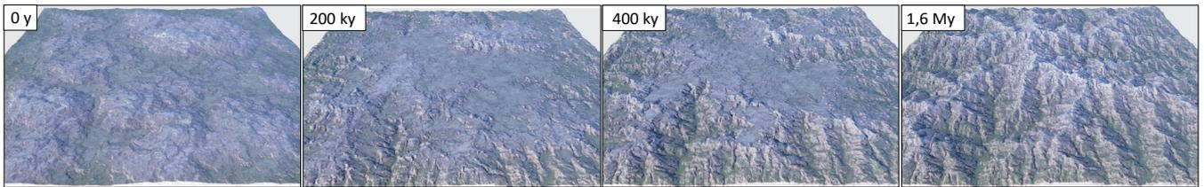
**Figure 1:** Our method receives as input an initial terrain ( $t = 0y$ , left), a map of the tectonic uplift, and a time  $t$ . Thanks to the analytical solutions of the stream power law, our method outputs the eroded terrain at time  $t$ , without the need of a costly simulation. Therefore, a user can easily explore the time continuum, from the early erosion of the input terrain ( $t = 200ky$ , center left) to the steady state equilibrium between uplift and erosion ( $t = 1.6My$ , right).
