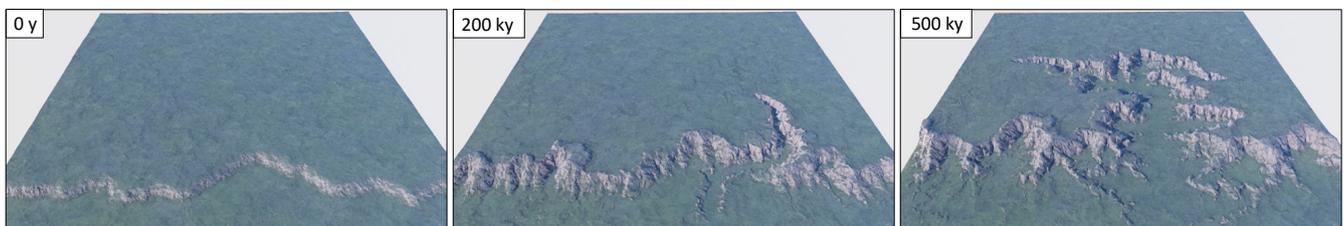
**Figure 12:** Evolution of a procedurally generated escarpment (left). After  $200ky$  the cliff retreats slightly and a canyon starts forming around the main river. After  $500ky$ , the canyon widens, inheriting the flat bottom from the lower part of the escarpment, and starts branching.
