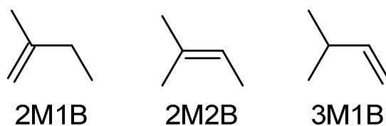
Figure 1: Chemical structures of the studied isomers. 2M1B: 2-methyl-1-butene, 2M2B: 2-methyl-2-butene, 3M1B: 3-methyl-1-butene.
