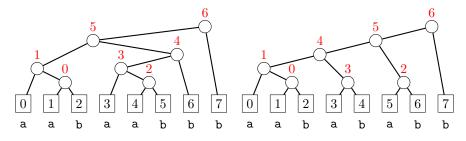
However with the permutation p = (1, 0, 5, 3, 2, 4, 6), the algorithm computes rank = (1, 0, 4, 3, 5, 2, 6) and the corresponding L tree (above right), which produces the word **aabababb**. But psp(aabababb) = (1, 0, 3, 2, 5, 4, 6) is not the input permutation. This is because obviously not all the (n - 1)! permutations are PSPs of some binary Lyndon words (less than  $2^n$ ). It may also happen that word y built in the procedure is not even a Lyndon word.
