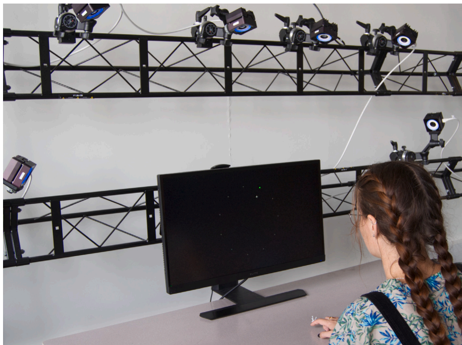
Fig. 1. The experimental setup. A participant is sitting at the desk, pointing with the index finger on the surface of the desk, and looking at the pointer and targets on the display. Optical tracking cameras are setup around the workspace. A small rigid body is attached to the index finger.
