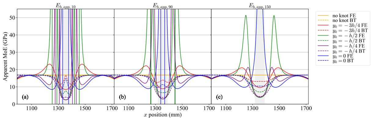
Fig. 9. Apparent MoE in bending obtained by FE (solid line) and BT modelling (dashed line) according to  $x$  position in the “5 times depth” central area of the beam, computed in 10 mm (a), 90 mm (b), and 150 mm (c) long sliding windows. [colour version online]
