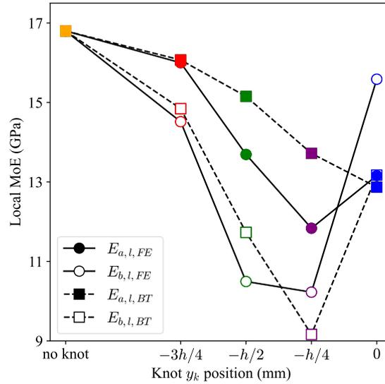
Fig. 10. Evolution of local MoE in axial loading (filled markers) and bending loading (empty markers) according to knot  $y_k$  position obtained by FE (solid line) and BT modelling (dashed line). The abscissa of the “no knot” beam has been set arbitrarily. Marker colours correspond to different knot  $y_k$  positions as in other Figures.
