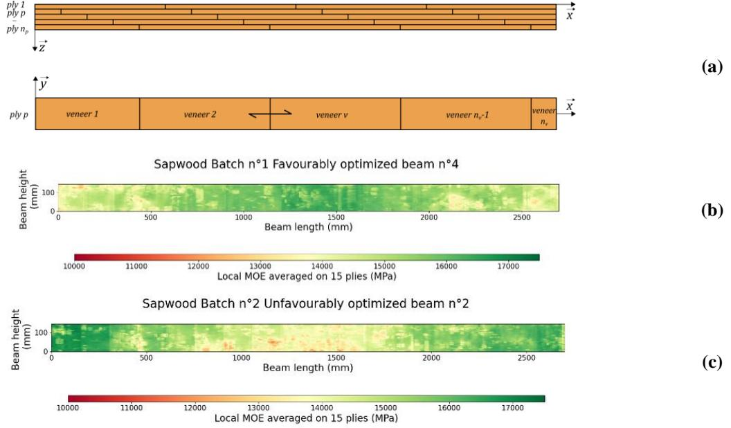
Fig. 2. (a) Schematical representation of the constitution of a LVL beam made of several plies ( $p$  index) and veneers ( $v$  index) (arrow represents main grain direction), (b) example of the modeled MoE repartition of a favourably optimized beam, borrowed from Duriot et al. (2021b), (c) example of the modeled MoE repartition of an unfavourably optimized beam, borrowed from Duriot et al. (2021b)
