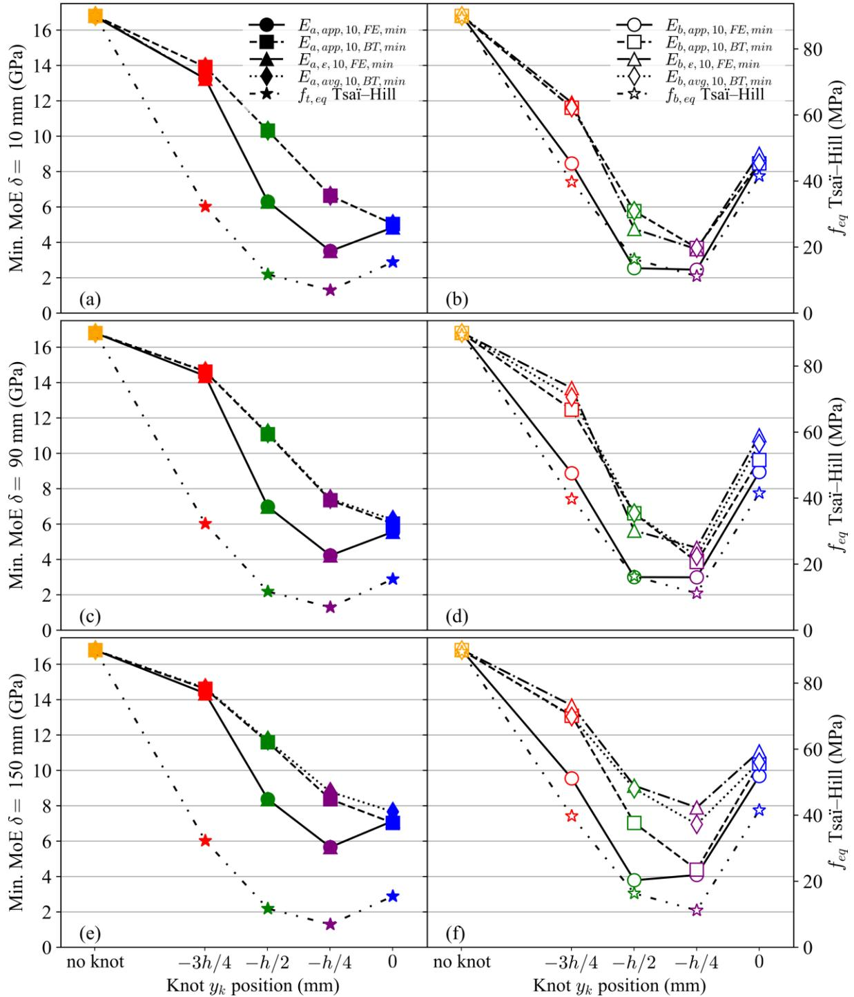
Fig. 14. Evolution of minimum localized MoEs and Tsai-Hill criterion for axial loading (filled markers, on the left) and bending loading (empty markers, on the right) according to knot  $y_k$  position obtained by different modelling methods, with sliding windows lengths of 10 mm (a,b), 90 mm (c,d), and 150 mm (e,f). Tsai-Hill criterion second axis scale has been set to be proportional to the apparent MoE for the homogeneous beam.
