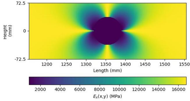
Fig. 4.  $E_x$  around knot area for an artificial beam with a knot centred in the beam depth
