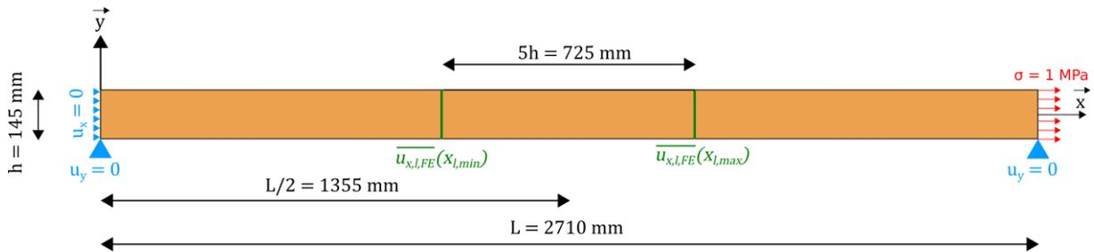
Fig. 5. Boundary conditions for FE axial loading
