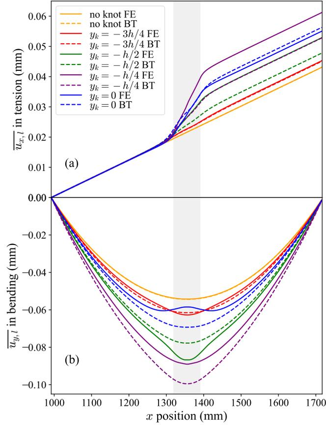
Fig. 7. Displacements averaged over beam depth ( $y$ -direction) obtained by FE (solid line) and BT modelling (dashed line) according to  $x$  position in the “5 times depth” central area of the beam, under axial tensile loading of 1 MPa (a), and a bending moment corresponding to a maximum stress of 1 MPa (b). Line colours refer to knot  $y_k$  position, the central grey rectangle represents the location and width of the knot (whose diameter was 72.5 mm). [colour version online]
