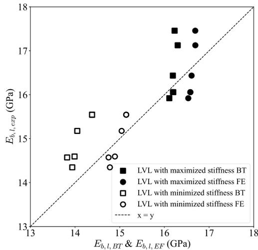
Fig. 11. Comparison between BT and FE bending local MoE versus experimental local MoE for each LVL beam
