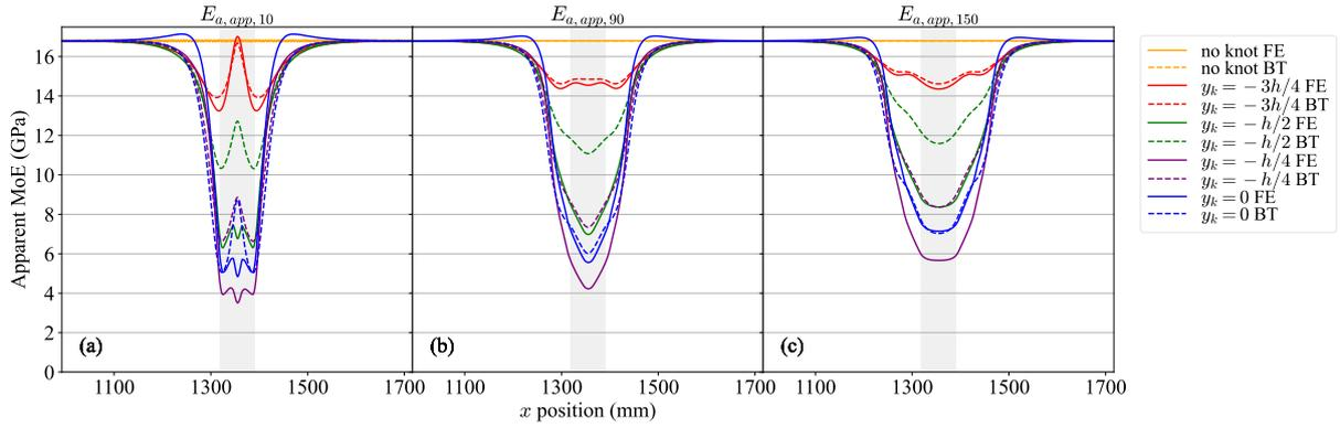
Fig. 8. Apparent MoE under axial loading obtained by FE (solid line) and BT modelling (dashed line) according to  $x$  position in the “5 times depth” central area of the beam, computed in 10 mm (a), 90 mm (b), and 150 mm (c) long sliding windows. [colour version online]
