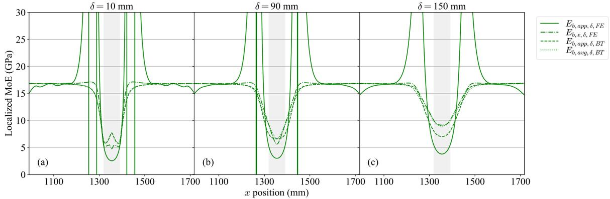
Fig. 13. Localized bending MoE comparisons in the case of the artificial beam with knot position  $y_k = -\frac{h}{2}$ , according to  $x$  position in the “5 times depth” central area of the beam and sliding-window lengths  $\delta$  of 10 mm (a), 90 mm (b), and 150 mm (c).
