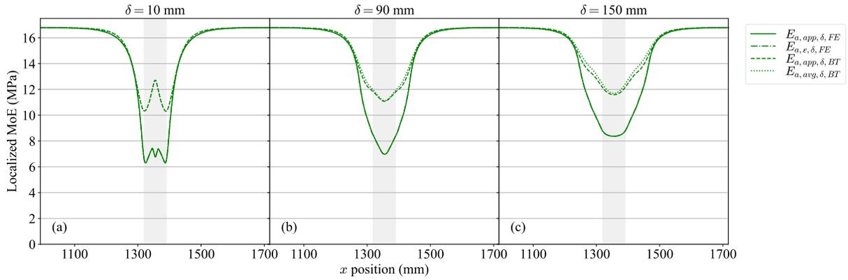
Fig. 12. Localized axial MoE comparisons in the case of the artificial beam with knot position  $y_k = -\frac{h}{2}$ , according to  $x$  position in the “5 times depth” central area of the beam and sliding-window lengths  $\delta$  of 10 mm (a), 90 mm (b), and 150 mm (c). Note that  $E_{a,app,\delta,FE} = E_{a,\epsilon,\delta,FE}$ , therefore the curves are indissociable.
