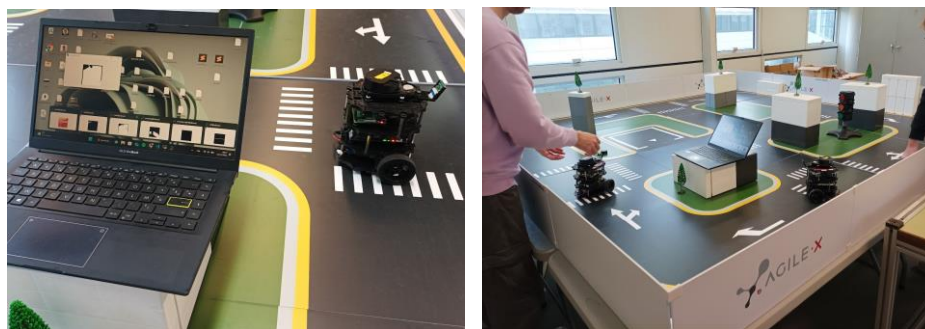
Fig. 5 In situ validation and tests of system behavior. The robot must perform autonomous navigation task in hard lighting conditions making IA model road recognition complex problem requiring a deep neural network challenging computing resources as well as system robustness.
