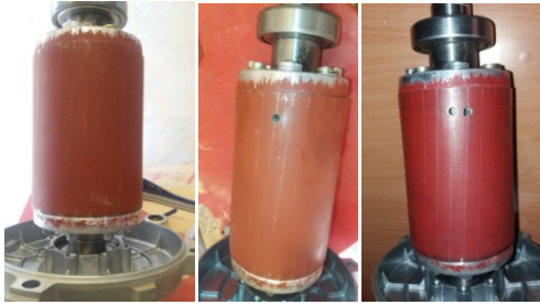
Fig. 2 Rotors photos (healthy and faulty rotor).
