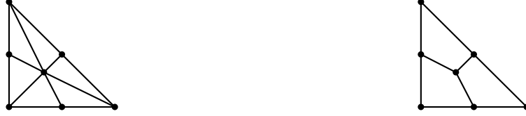
(a) The barycentric subdivision of a triangle. (b) The cubical subdivision of a triangle.
