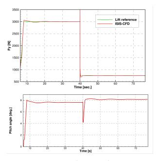
Fig. 7. Cl = 1.4,  $U_{\infty}$  = 56.7 ms<sup>-1</sup> to 28.4 ms<sup>-1</sup>: Evolution of lift force (top) and pitch angle (bottom) versus the time
