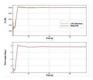
Fig. 5.  $F_y^* = 3000$  N, Re =  $4.70 \times 10^6$ ,  $U_{\infty} = 56.7$ . ms<sup>-1</sup>: Evolution of lift force (top) and pitch angle (bottom) versus the time
