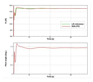
Fig. 4.  $F_y^*=1500$  N, Re =  $4.70\times10^6$ ,  $U_\infty=56.7$ . ms $^{-1}$ : Evolution of lift force (top) and pitch angle (bottom) versus the time
