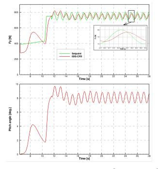
Fig. 11. Sinusoidal  $F_y^*$  (f=1 Hz), Re =  $2.35\times10^6$ ,  $U_\infty=28.4$  ms $^{-1}$ : Evolution of lift force (top) and pitch angle (bottom) versus the time
