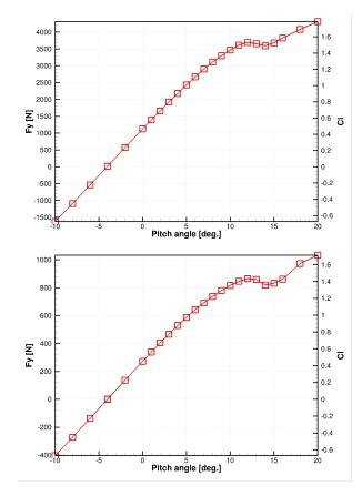
Fig. 3. Evolution of lift force and lift coefficient versus the pitch angle for two Reynolds numbers Re =  $4.70\times10^6$ ,  $U_{\infty}$  = 56.7. ms $^{-1}$  (top) and Re =  $2.35\times10^6$ ,  $U_{\infty}$  = 28.4. ms $^{-1}$  (bottom)
