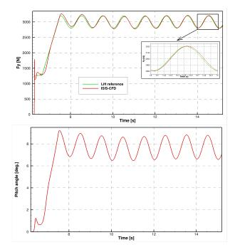
Fig. 10. Sinusoidal  $F_y^*$  (f=1 Hz), Re = 4.70×10<sup>6</sup>,  $U_\infty$  = 56.7 ms<sup>-1</sup>: Evolution of lift force (top) and pitch angle (bottom) versus the time
