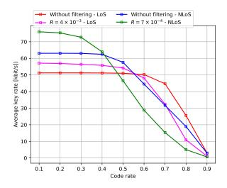
Fig. 7. Average key rate for LoS and NLoS conditions considering different code rates and filtering paratemers.
