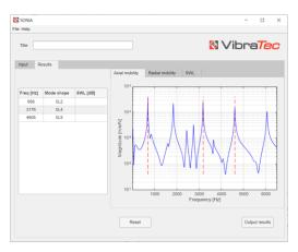
**Figure 7**. SONIA application – wheel damping.
