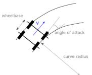
Figure 1: Railway curve negotiation.
