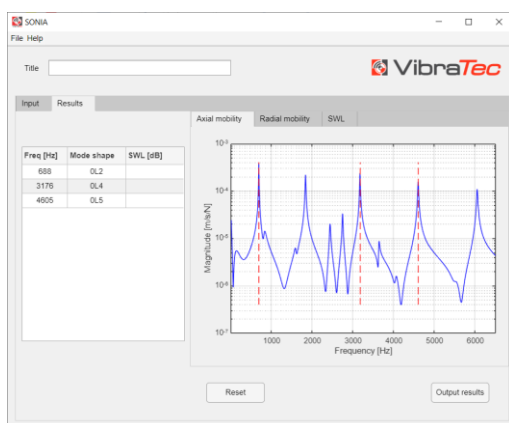
Figure 7. SONIA application – wheel damping.
