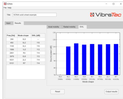
**Figure 5.** SONIA interface: outputs - sound power.
