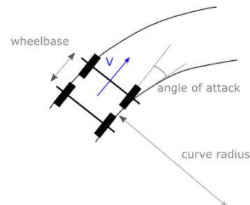
**Figure 1:** Railway curve negotiation.
