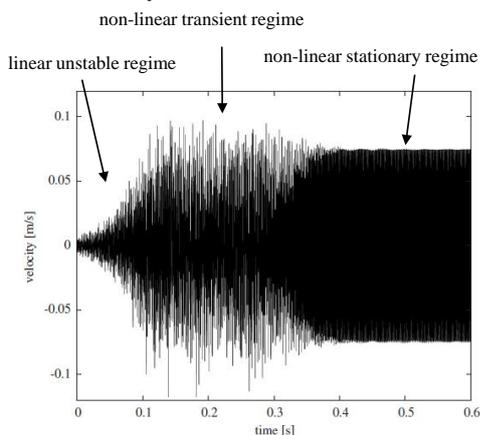
**Figure 2:** Typical time history of self-sustained vibrations [4].
