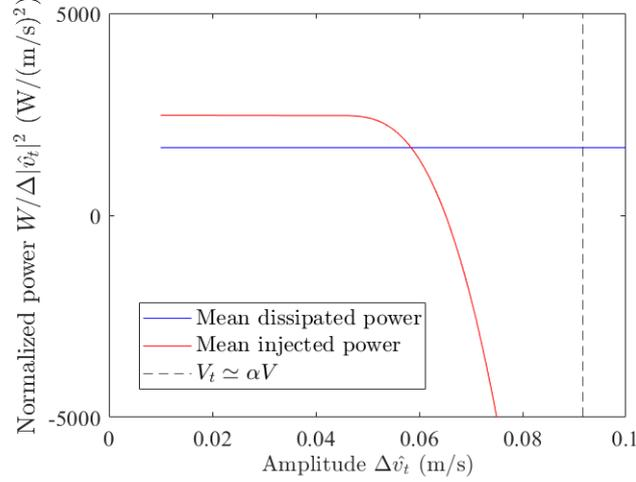
**Fig. 3.** Power balance as a function of the cycle amplitude for the reduced model
