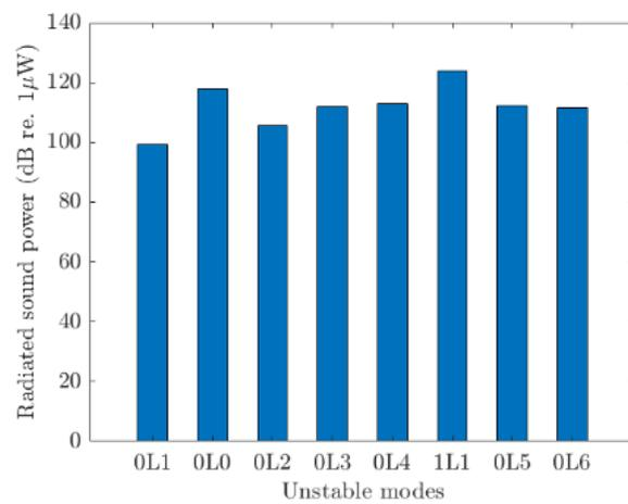
**Fig. 4.** Radiated sound power for each unstable mode
