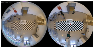
Fig. 5: Aranjuelo et al. [39] utilized 3ds Max software to virtually render humans (right) on a real scene (left) for detection of moving subjects.
