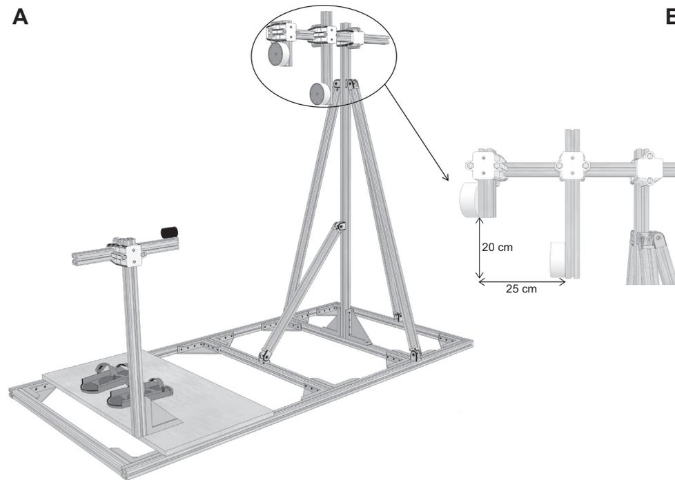
**Fig. 1.** Experimental setup. (A) Global view of the pointing structure including targets, start push-button (black array) and footstraps. (B) Side view of the targets which illustrates the position of the far target relative to the close target.
