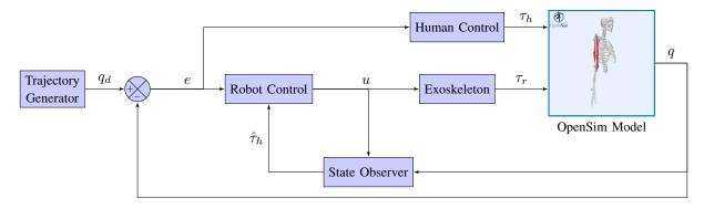
Fig. 1. Control block diagram of the system
