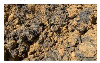
Figure 7: The two types of shale clays mixed in a factory in al-Rihawi (Egypt) © C. Pérez-Houis, March 2022
