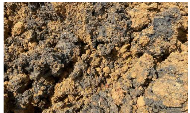
Figure 7: The two types of shale clays mixed in a factory in al-Rihawi (Egypt)
