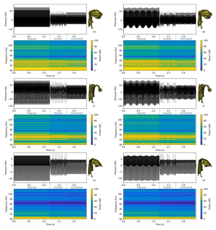
Fig. 9. Time evolution and spectrogram for vowels  $/\alpha$ , /i/ and /u/ in the regular, chaotic and controlled phonation regimes without vibrato. Access the supplementary material to listen to the corresponding audio files.
