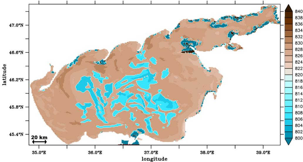
Figure 8: Average dry density of sediment (in  $\text{kg/m}^3$ ) at July 1st, 2021, with an initial mean over sediment thickness dry density set at  $347 \text{ kg/m}^3$ .
