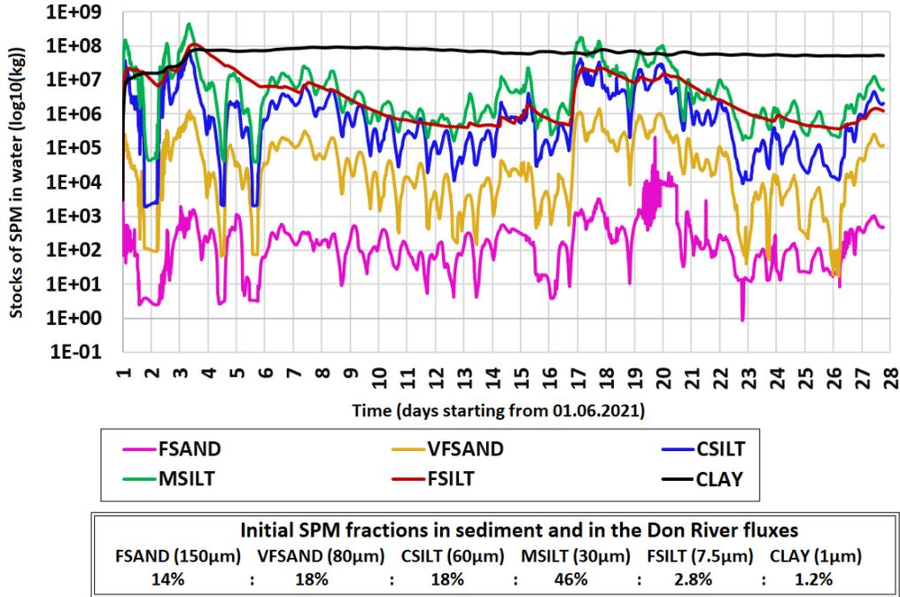
Figure 4: Time-evolution of the stocks in water of SPM ( $\log_{10}(\text{kg})$ ) in the Taganrog Bay area ( $38.75^{\circ}\text{N}$ - $39.3^{\circ}\text{N}$ ;  $48.75^{\circ}\text{E}$ - $47.3^{\circ}\text{E}$ , volume of approximately  $4 \text{ km}^3$ ).
