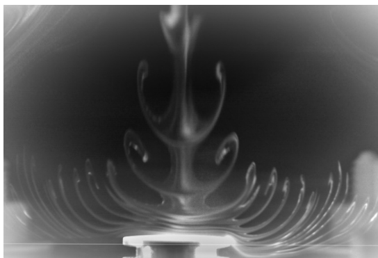
FIG. 11. Example of dust ejected by an atmospheric pressure Ar/HMDSO flow-through plasma and interacting with a witness sample for contamination control research (courtesy of T. J. A. Staps and T. J. M. Donders, CIMlabs, Eindhoven University of Technology, The Netherlands).
