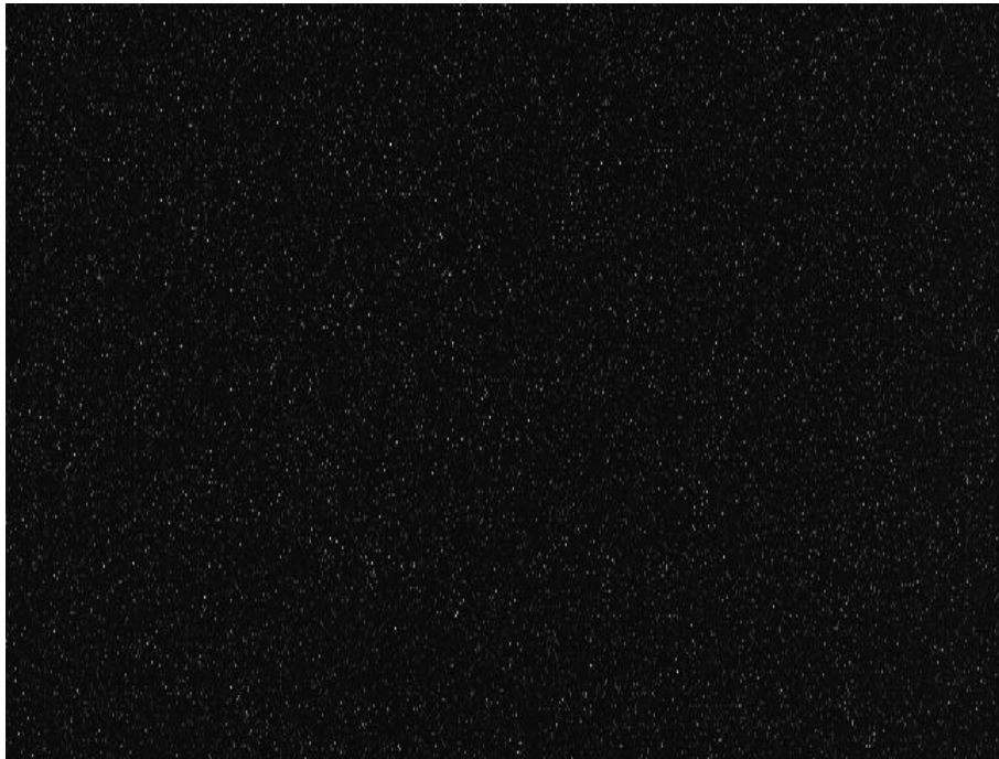
Figure 5 : Standard deviation image from a 0.35 micron VGA image sensor
