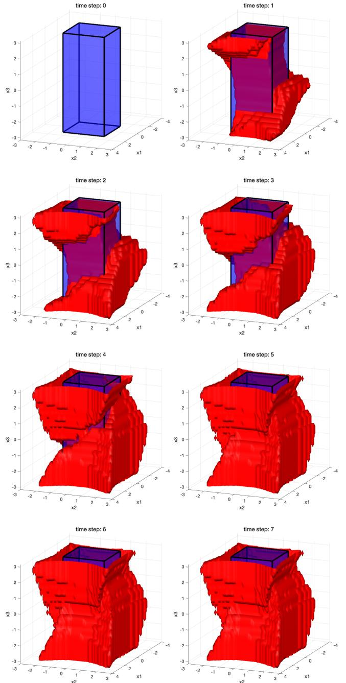
Figure 3: The evolution of the set  $\text{CPre}_{[1:K]}$  (red parts) with  $K$  is depicted in the figure, where  $K = 0, 1, 2, \dots, 7$ . By the fifth iteration step, the hyperrectangle is completely contained in the computed states, and by the seventh iteration step, the computed states are identical to the maximum control invariant set.
