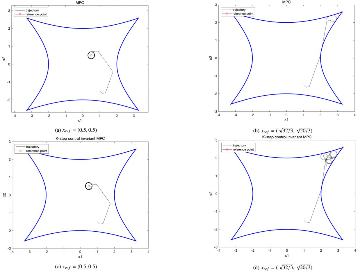
Figure 4: Trajectory of moving carts. The upper two figures show the NMPC approach without terminal constraints and the two figures below show the NMPC using a  $K$ -step control invariant set ( $K=5$ ) as terminal constraint.
