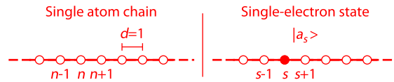
FIG. 16. (a) Representation of the chain of atoms, where each atom is identified by the running label n = \{\dots, -1, 0, 1, \dots\} and the lattice parameter is taken as 1. (b) Representation of the single-electron state |a_s\rangle , which corresponds to a state where a single electron is localized on atom s .
