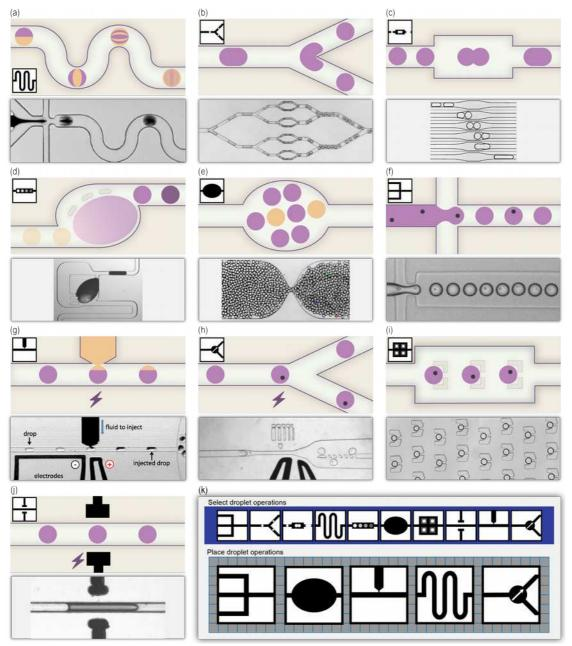
Figure 2 Droplet manipulations and unit operations.
