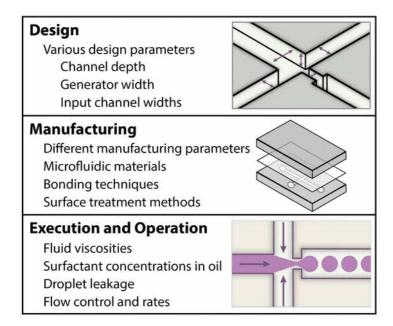
Figure 7 Summary of sources of variability in droplet-based microfluidic experimentation.
