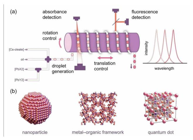
Figure 6 Droplet-based microfluidic synthesis of materials with bespoke properties.
