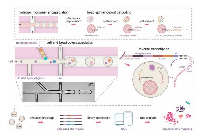
Figure 4 Droplet-based single-cell RNA sequencing (scRNA-seq).
