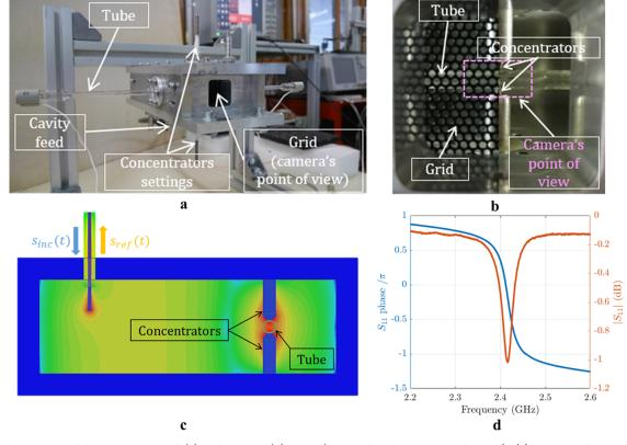
Figure 1. Photographs of the cavity. External (a) and internal (b) views (with and without the Faraday grid). (c) Numerically simulated E-field profile of the  $TE_{012}$  mode. (d)  $S_{11}$  as a function of frequency, measured with a vector network analyzer.
