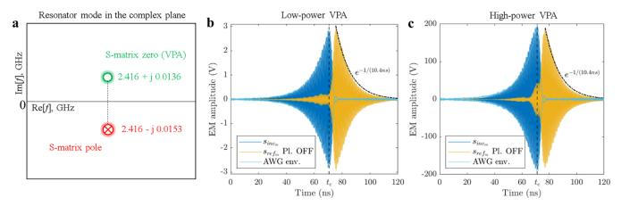
**Figure 2.** (a) Experimentally deduced position of the pole and zero of the resonant mode under consideration. Low-power (b) and high-power (c) VPA without plasma: measurements of the incident and reflected microwave signal amplitudes with the oscilloscope (no plasma, 500  $\mu$ s repetition period). These results are averaged over 64 measurements. The raw signal captured on the oscilloscope for a single pulse is provided in the Supporting Information.
