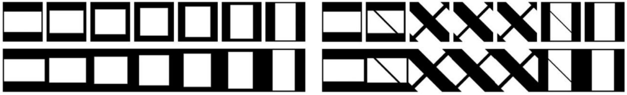
(a) Micro-structures obtained for density = 0.5, orientation angle \alpha = 0 rad and extended cubicity values ranging from 0.2 to 0.8. (b) Micro-structures obtained for density = 0.5, orientation angle ranging from 0 rad to \pi/2 rad and extended cubicity equals to 0.2.
