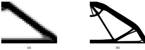
Fig. B1. Comparison of half MBB designs. a top88 design on a 32 \times 24 grid and b top88 design on a 800 \times 600 grid.
