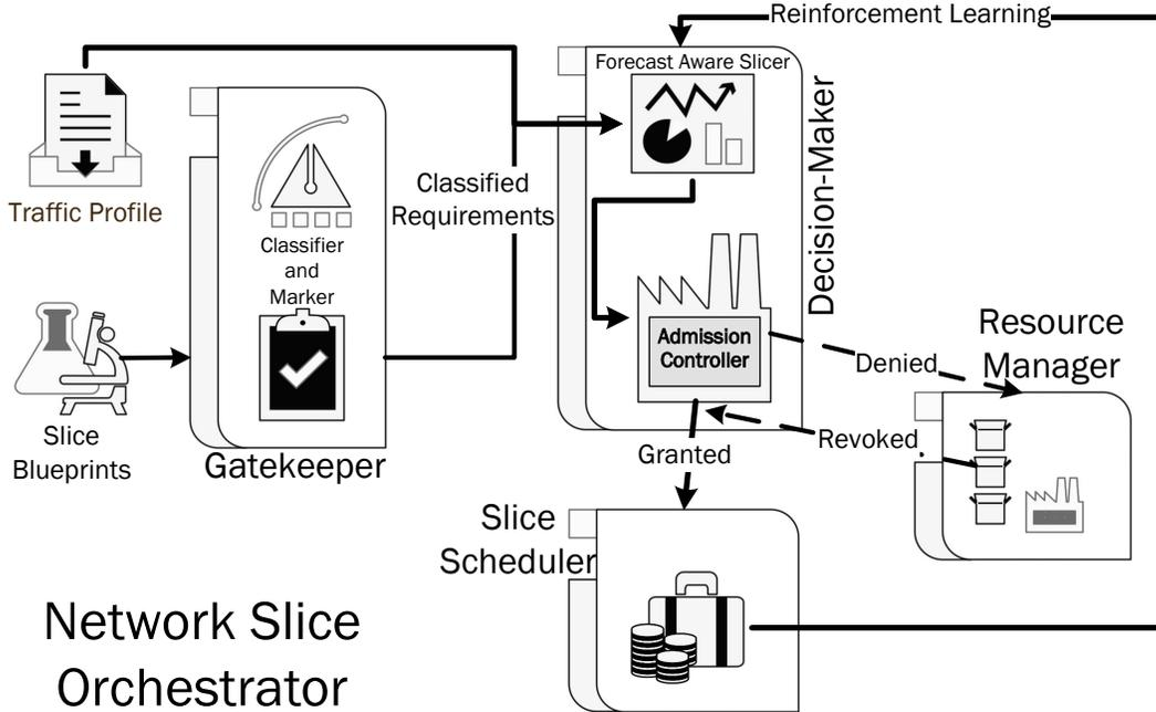
Figure 1: Block Diagram of 5G Network Slice Orchestrator
