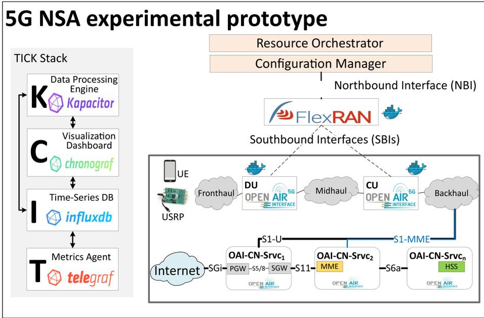
Figure 3: Our 5G experimental prototype block diagram
