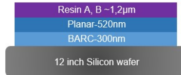
Figure 4. Diagram of resists stack for grayscale lithography
