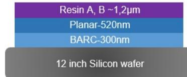
Figure 4. Diagram of resists stack for grayscale lithography
