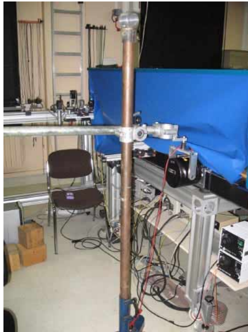
Fig. 2. Picture of the experimental set-up for vibration filtering validation. The AO bench is on the right, under its baffling. The seismic vibration generator is in the middle of the picture, placed on its stage and against the AO bench (cylindrical black component).
