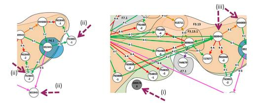
Figure 8. Most recurrent errors in product modelling: (i) isolated components, (ii) no functional allocation, (iii) redundant components.
