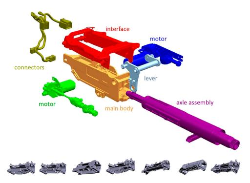
Figure 7. Main subassemblies of a steering column and an example of variant components below.
