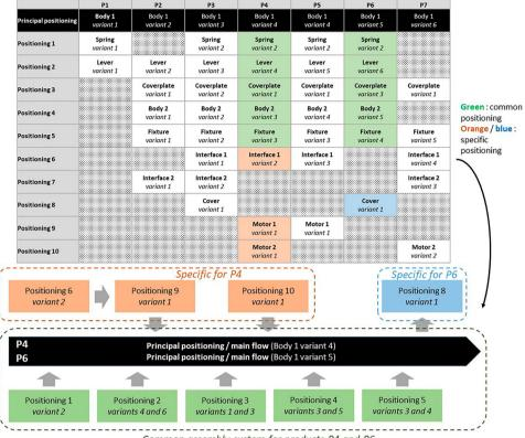
Common assembly system for products P4 and P6
