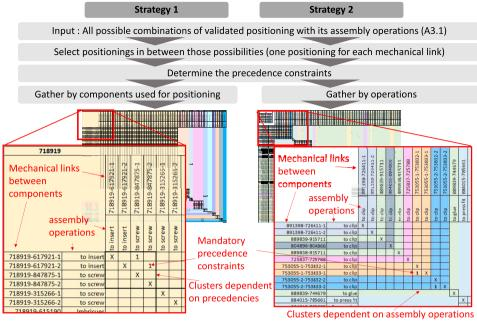
For both matrices : same colour = same component used for positioning during assembly
