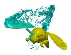
**Figure 9.** Visualization of flow generated by a tethered flapping bumblebee with flexible wings in laminar flow at Re = 2685 showing normalized absolute vorticity isosurfaces  $|\underline{\omega}| = 100$  (light blue). The flow field is plotted at time t/T = 0.45. The vortices are only shown in the right half of the computational domain for the purpose of visualizing the deformation of the left wing. Adapted from [64].
