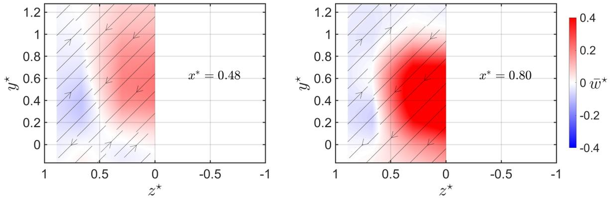
Figure 9: Rear view of the 2D mean maps of the dimensionless transverse velocity and the streamlines associated behind the LV  $\varphi = 25^\circ$  for  $d^* = 0.93$  in the planes  $x^* = 0.48$  and  $x^* = 0.80$ .
