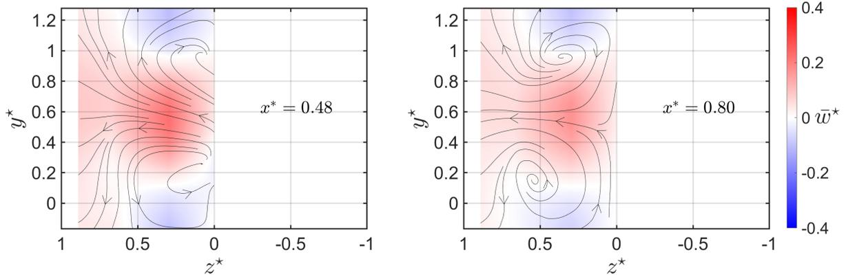
Figure 7: Rear view of the 2D mean maps of the dimensionless transverse velocity and the streamlines associated behind the LV  $\varphi = 0^\circ$  for  $d^* = 0.93$  in the planes  $x^* = 0.48$  and  $x^* = 0.80$ .
