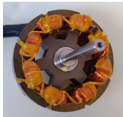
Figure 1: Manufactured SR motor - wound stator, rotor and shaft.
