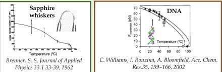
Traditional fracture mechanics results (energy release rate, fracture toughness, and J-integral) are extended to incorporate temperature effects.
