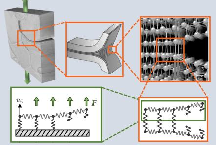
A **microscopic** model for fracture propagation has been formulated. The crack propagation is described by employing a **discrete** model made of a succession of n units. Each unit is modeled as an elastic spring and a breakable element that can switch from an attached to a detached state once the fracture threshold is reached.
