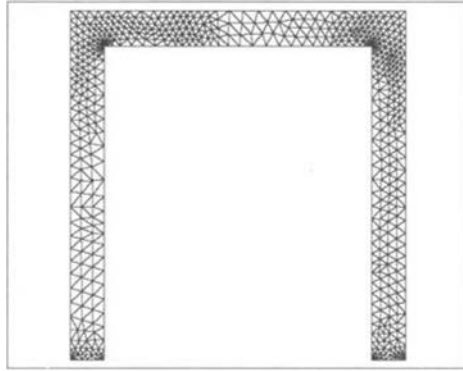
Figure 25. Final mesh optimized with Drucker error, 1286 six-node triangles, 12 time steps
