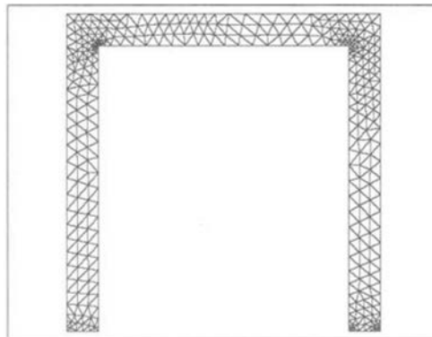
Figure 24. Final mesh optimized with the dissipation error, 661 six-node triangles, 11 time steps
