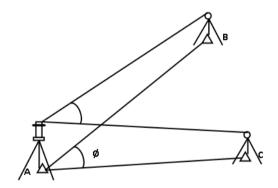
Fig. 3. In situ check with a total station
