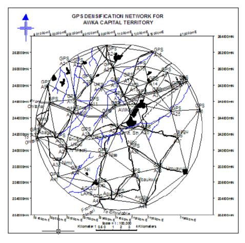
Fig. 2. Network of control stations in Awka
