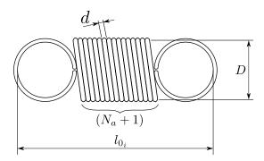
Figure 5: Schematic of a helical extension spring.
