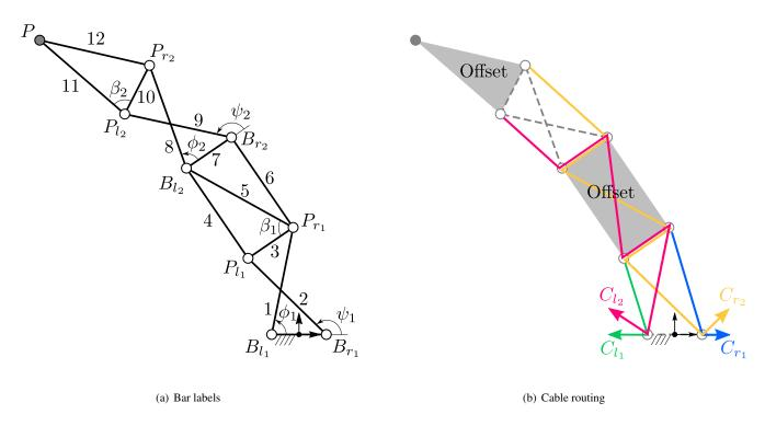
Figure 2: Bar labels (left) and cable routing scheme (right) for the 2-X manipulator.
