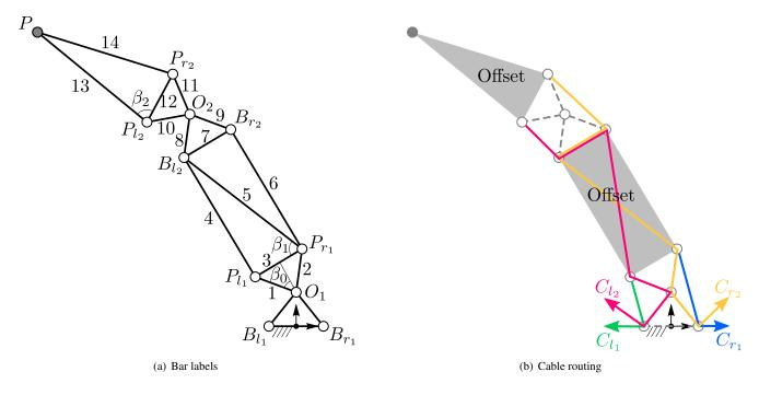
Figure 10: Bar labels (left) and cable routing scheme (right) for the 2-R manipulator.
