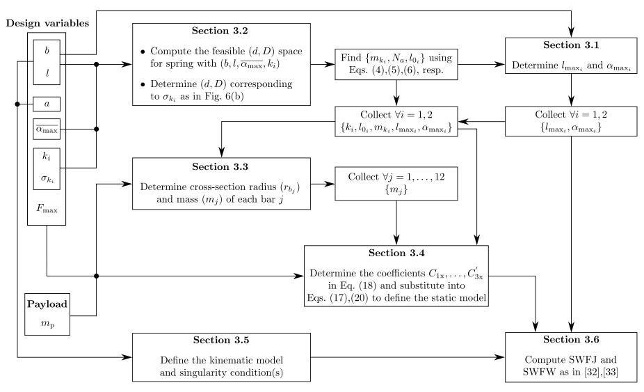
Figure 8: Computational scheme for the determination of SWFW for the 2-X manipulator that accounts for all of its design considerations discussed in Section 3.
