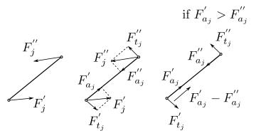
Figure B.14: Computation of the buckling load in the bar j subjected to forces  $F'_j$  and  $F''_j$  at the two ends.
