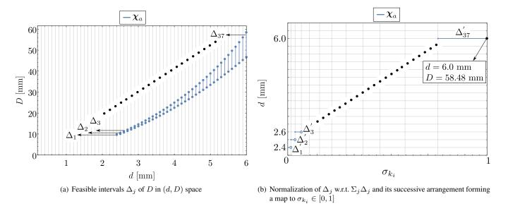
Figure 6: Parametrization of the feasible spring space with  $\sigma_{k_i} \in [0,1]$  when  $k_i = 3000$  N/m for an X-joint with b = 0.2 m and l = 0.4 m, and  $\overline{\alpha_{\max}} = 5\pi/6$  rad.
