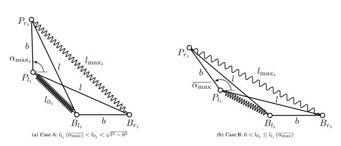
Figure 4: Joint limits of an X-joint depending on the spring free length and bar lengths.
