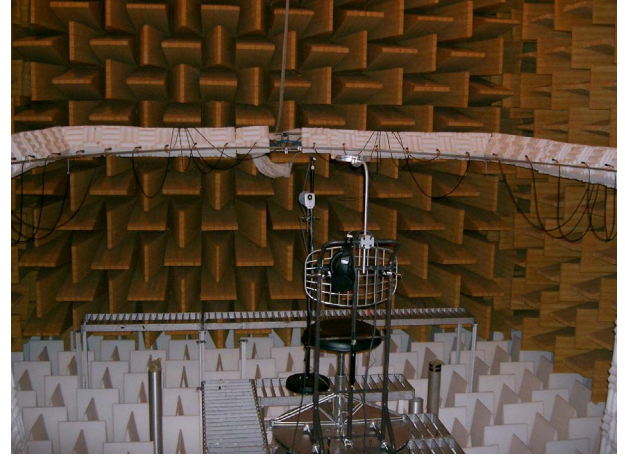
Figure 1. Directivity measurement system including the rotating arc, reference microphone and rotating chair.
